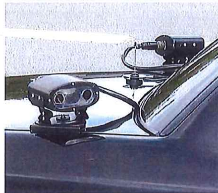
Photo 8 - Sample LPR Installation
