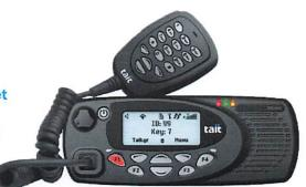
The TM9400 is capable of AES encryption, Over-the-air Rekeying (OTAR), various emergency modes and is IP54 rated to keep those relying on the mobiles safe and efficient. The TM9400 also has an options slot allowing extension of capabilities and a range of remote mounting and control head options.
