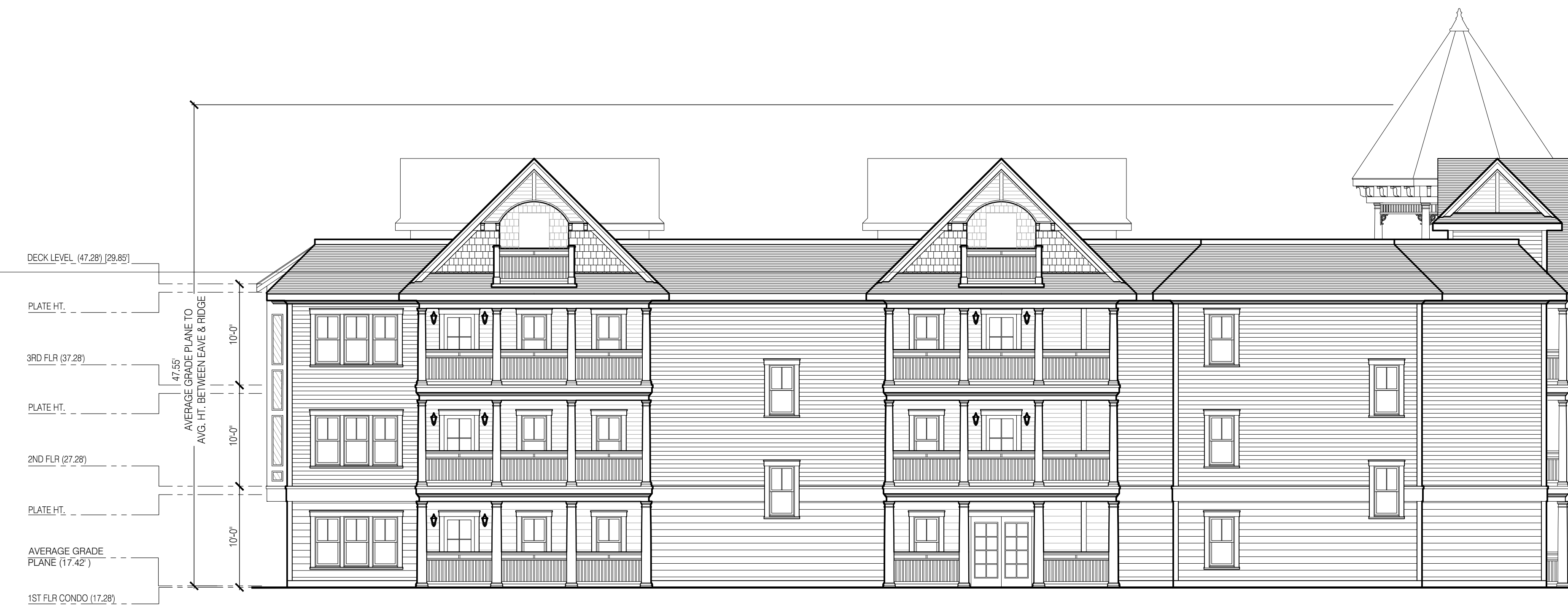
④ BUILDING 2 - SOUTH ELEVATION 1/8"=1'-0"
