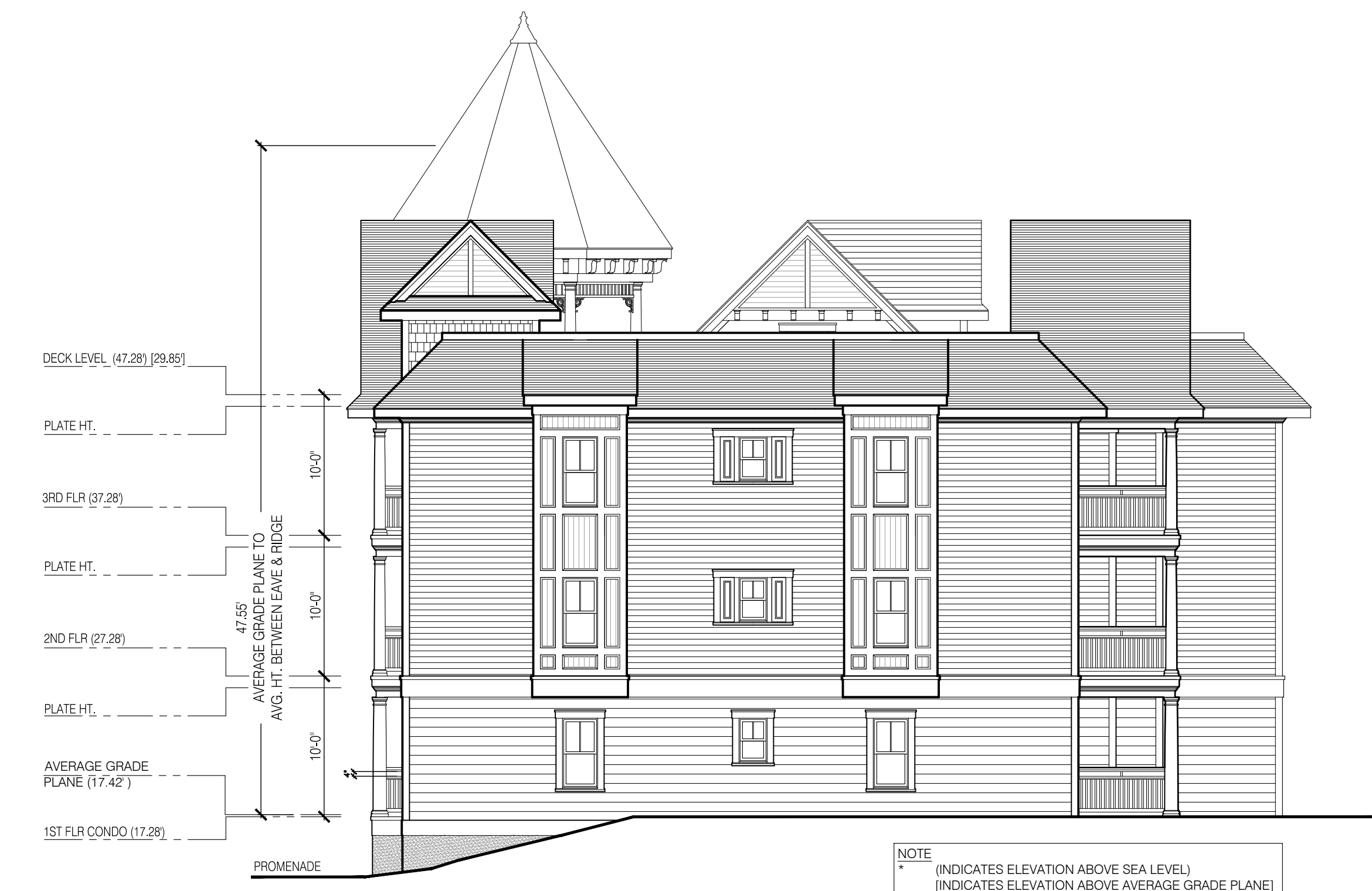
③ BUILDING 2 - WEST ELEVATION 1/8"=1'-0"
