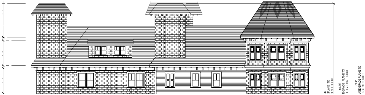
Illustration C.8.d. — Hotel dormers, west elevation, showing two sets of double windows beneath a shed roof (Sheet A-12).
