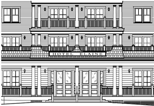
Illustration D.2. — The south elevation (Sheet A-11) showing proposed double set of double \frac{1}{2} doors, with non-conforming single side-light windows to the left and right.
