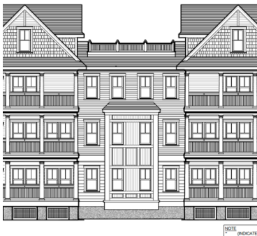
Illustration F.5.b. — Detail of north elevation, Condominium Building Two, showing paneled areas between windows on projection between balconies (Sheet A-8).
