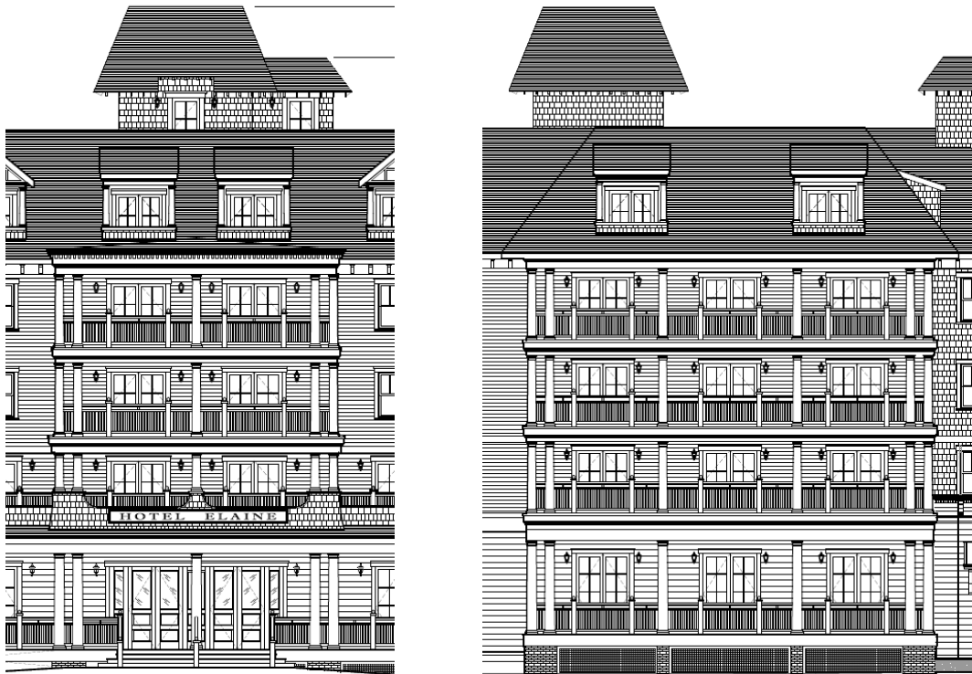
Illustration H.2.a. and H.2.b. — Details of the balcony stacks at the south and east elevation of the Hotel showing double and single columns and newels (Sheet A-11).
