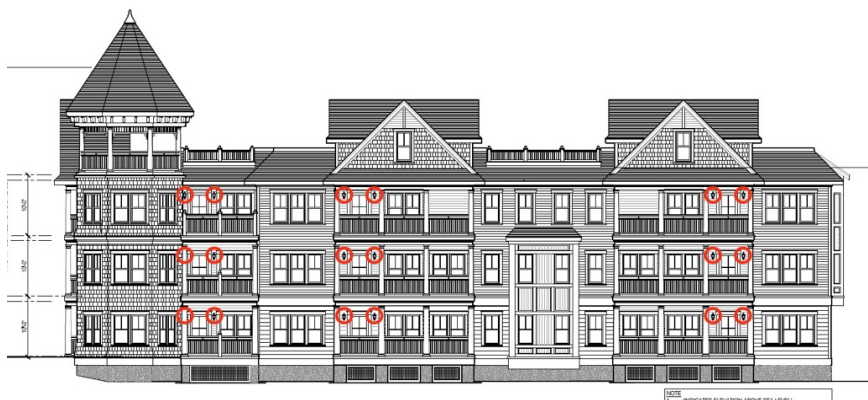
Illustration I.8.b. — North elevation of Condominium Building Two showing lighting (all of which entails two light fixtures flanking single doors onto balconies) (Sheet A-8).
