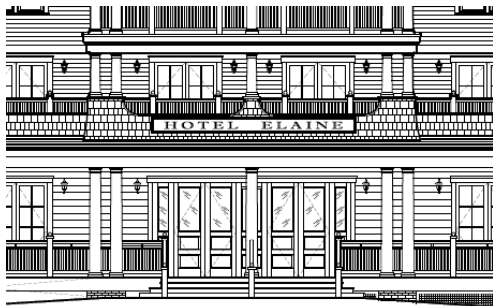
Illustration H.1. — Hotel entrance flanked by double columns with single column bisecting the entry area (Sheet A-11).
