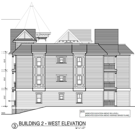
Illustration F.5.c. — Detail of west elevation, Condominium Building Two, showing paneled areas between windows on projections (Sheet A-8).
