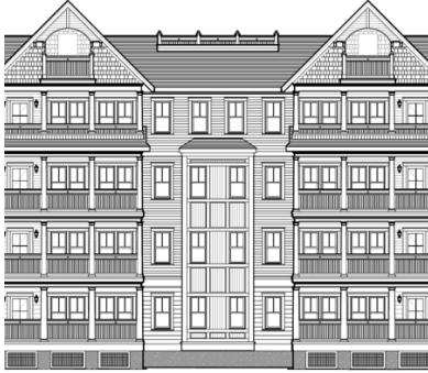
Illustration F.5.a. — Detail of north elevation, Condominium Building One showing paneled areas between windows on projection between balconies (Sheet A-6).
