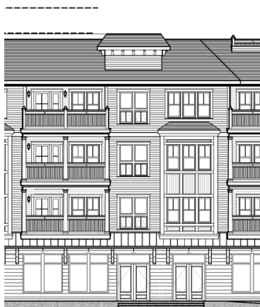
Illustration E.7. — Detail of staircase windows (center) configured in such a way as to suggest 2/1 windows have been installed upside down (Sheet A-5).
