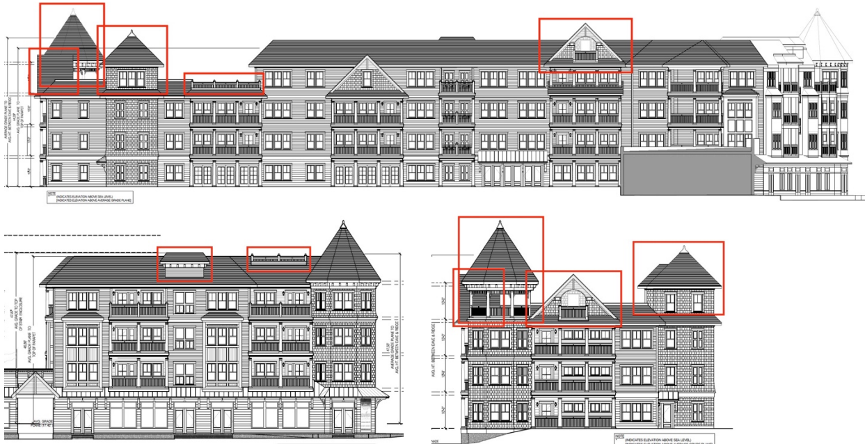
Illustrations C.14.a., C.14.b., C.14.c., and C.14.d. — The north, south, east, and west elevations of Condominium Building One showing non-conforming faux-gables, balusters and rails, cupola, and stair towers (Sheets
