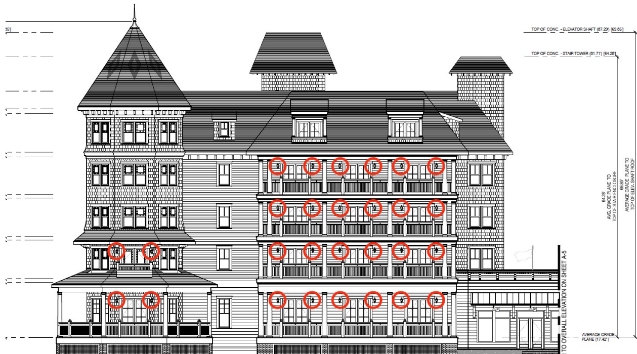
Illustration I.4.b. — East elevation of the Hotel showing twenty-eight (28) proposed lantern fixtures (Sheet A-11).
