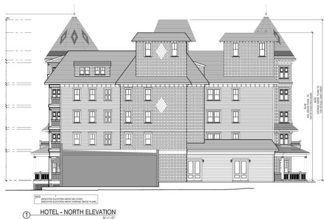
Illustration F.4. — North elevation of the Hotel showing over-sized diamond patterns in shingled cladding. (Sheet A-12).
