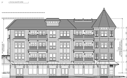
Illustration D.4. — East elevation of Condominium Building One (Sheet A-5) showing single balcony doors with non-conforming single side-light windows on each of the six balconies. These balcony doors should match single balcony doors on other elevations and should not include side-light windows.
